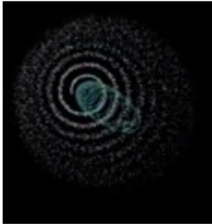
ALL PARTICLES IN THIS SPIRAL ARE MOVING RADIALLY OUTWARDS FROM THE AXIS OF MISSILE FLIGHT. THEY ARE **NOT** SPINNING AROUND THAT AXIS.
