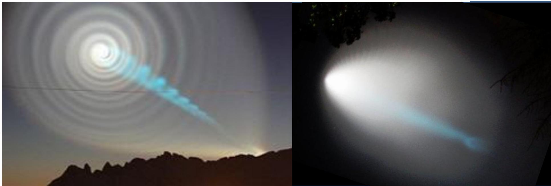
BOTH IMAGES SHARE WHITE PLUME OF MAIN ENGINE EFFLUENT AND A NARROWER BLUE PLUME POSSIBLY FROM THE HYDRAZINE-FUELLED HYDRAULIC POWER UNIT [HPU] NEEDED TO SWIVEL THE ENGINE NOZZLE [UNDER NEARLY IDENTICAL SOLAR BACKLIT ILLUMINATION CONDITIONS]. MUCH SLOWER PLUME EJECTION SPEED FROM HPU VERSUS ENGINE CREATES THE MUCH NARROWER PLUME SPREAD PATTERN AS OBSERVED.
